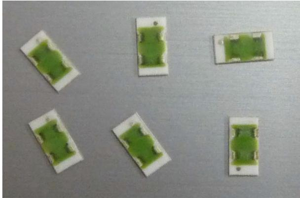
Typical Ceramic Strain Gauge
